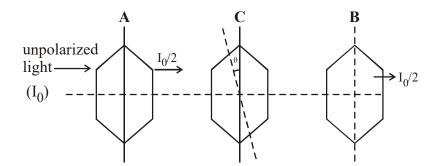
Here from both A and B, intensity becomes  $\frac{\omega}{2}$  so both have parallel pass axis.
