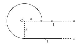
An infinite wire has a circular bend of radius a, and carrying a current I as shown in figure. The magnitude of magnetic field at the origin O of the arc is given by:
