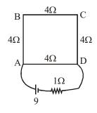
Equivalent resistance of the circuit =  $3 + 1 = 4 \Omega$
