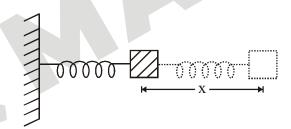
The equation of motion is given by  $x(t) = A\sin\omega t + B\cos\omega t$  with  $\omega = \sqrt{\frac{K}{m}}$  Suppose that at time t = 0, the position of mass is x(0) and velocity v(0), then its displacement can also be represented as  $x(t) = C\cos(\omega t - \phi)$ , where C and  $\phi$  are:
