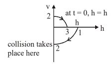
$1 \rightarrow 2$ : V increases downwards At  $2 \rightarrow$  velocity changes its direction  $2 \rightarrow 3$  V decreases upwards
