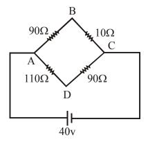
In the given circuit calculate the potential difference between points A and B
