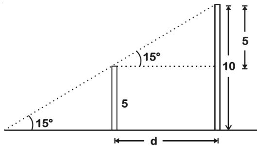
$$\begin{aligned}\tan 15^\circ &= \frac{5}{d} \Rightarrow d = \frac{5}{\tan 15^\circ} = \frac{5(\sqrt{3} + 1)}{\sqrt{3} - 1} \\ &= \frac{5(4 + 2\sqrt{3})}{2} \\ &= 5(+2\sqrt{3})\end{aligned}$$
