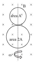
(A) The amplitude of the maximum net emf induced due to both the loops is equal to the amplitude of maximum
