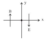
Force due to electric field is along –y axis and force due to  $\vec{B}$  is zero.
