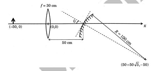
If the origin of the coordinate system is taken to be at the centre of the lens, the coordinates (in cm) of the point (x, y) at which the image is formed are -
